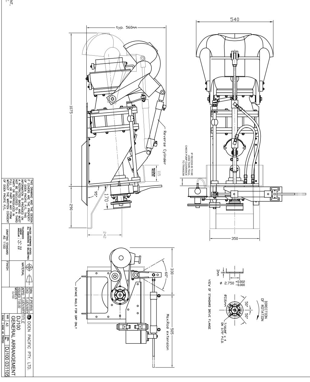
STANDARD MOULD INSERT PROVIDES FOR A MAXIMUM RECESS OF 115mm, SHOULD A RECESS GREATER THAN 115mm BE REQUIRED THE MOULD INSERT HEIGHT WILL NEED TO BE INCREASED TO CLEAR THE REVERSE RAM'S FWD. BRACKET
